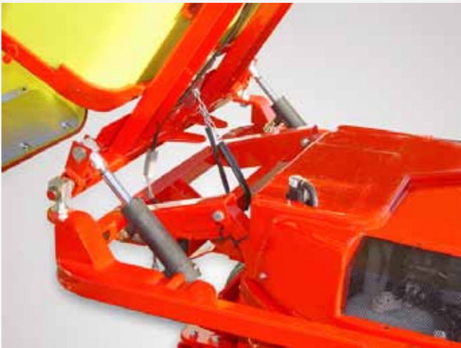
SportChamp SC2B/D: Hydraulic lifting for tipping the filter box
