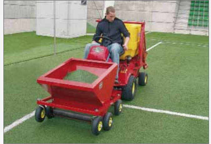
Sand / Rubber spreading device
